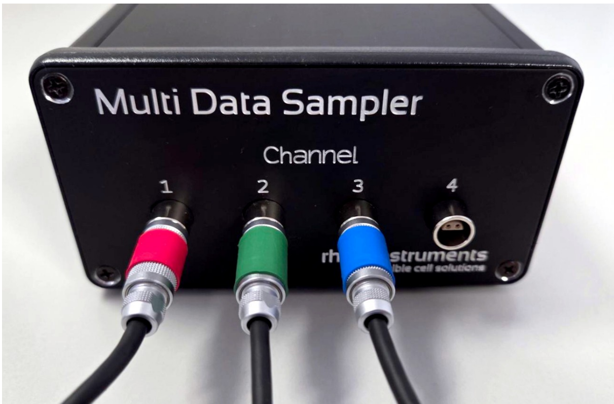
Figure 7: Connect the sensors to the RHD Multi Data Sampler. Connect the Multi Data Sampler to the computer using RS-232 or USB via the adaptor, connect the 24V DC power supply and switch on.
