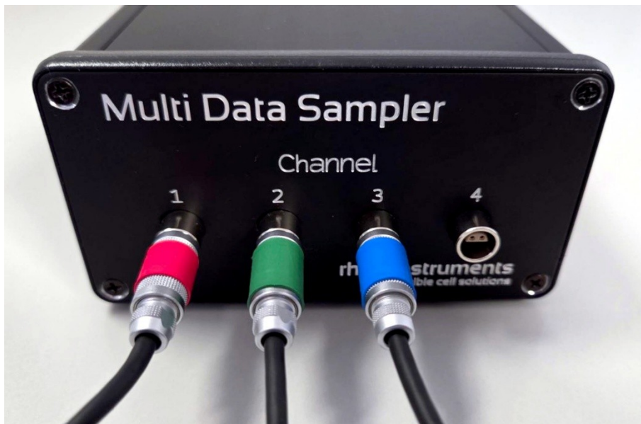
Figure 28: Connect the sensors to the RHD Multi Data Sampler via the 4-pin LEMO connectors. Connect the Multi Data Sampler to the computer using RS-232 or USB via the adaptor, connect the 24V DC power supply and switch on.
