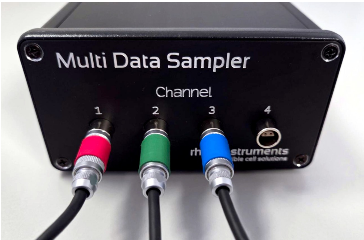
Figure 7: Connect the sensors to the RHD Multi Data Sampler via the 4-pin LEMO connectors. Connect the Multi Data Sampler to the computer using RS-232 or USB via the adaptor, connect the 24V DC power supply and switch on.
