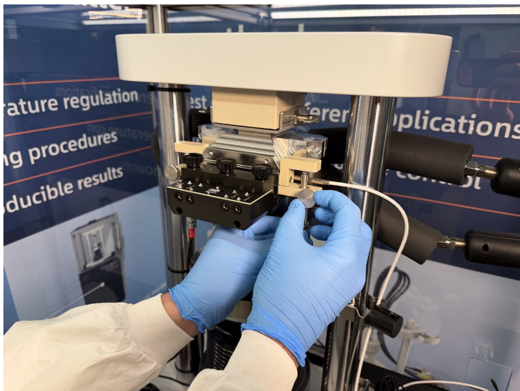
Figure 31: Fix the sensor in place by tightening the thumb screw. Do not overtighten.
