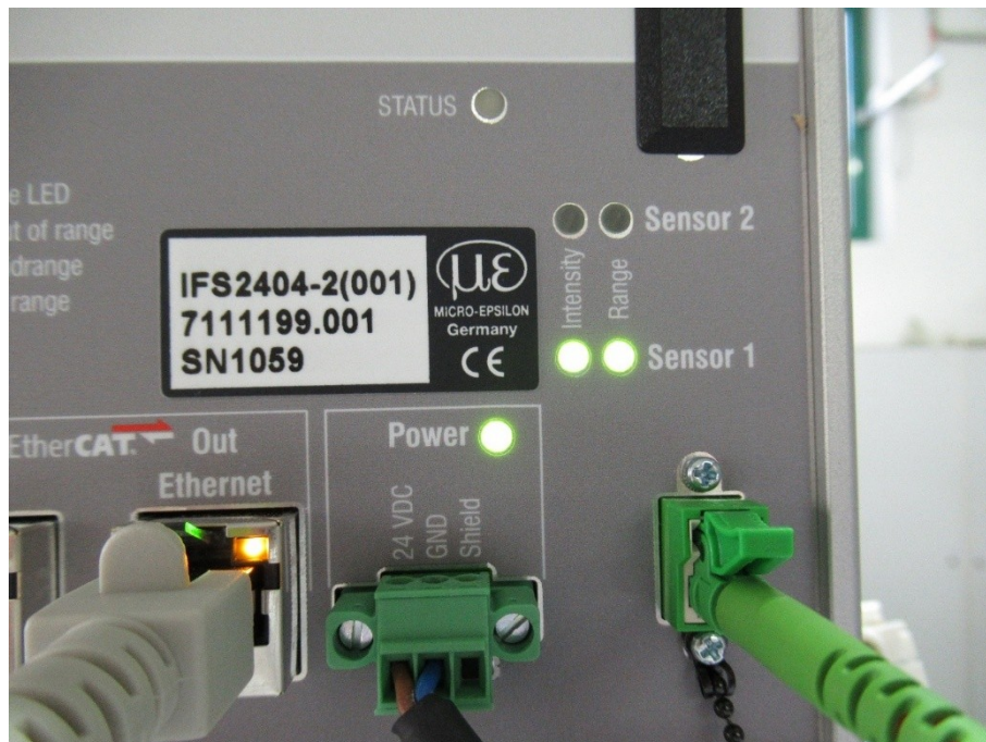
Figure 18: Sensor LEDs on the sensor controller.
