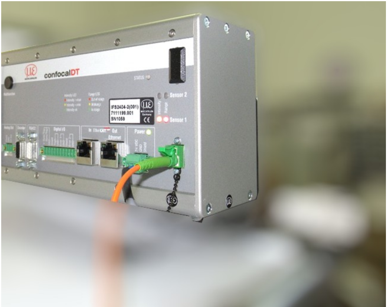
Figure 5: Sensor cable inserted into the sensor port of the controller
