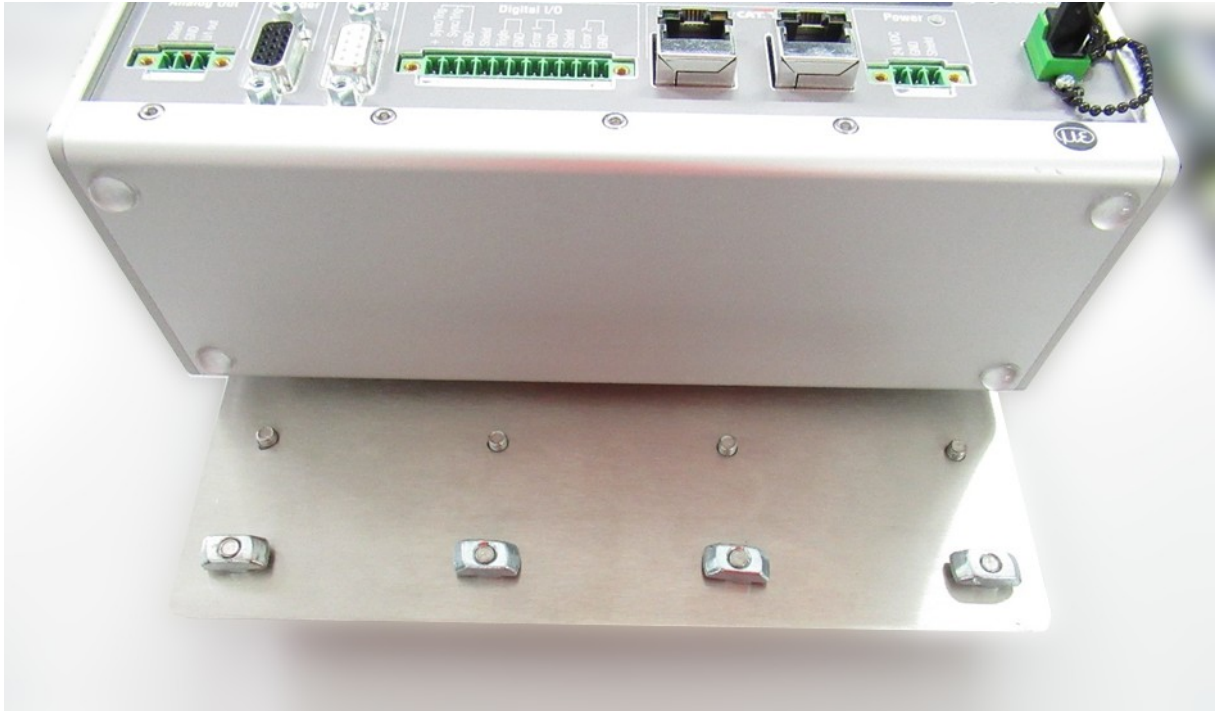
Figure 2: Confocal controller on support plate with aligned sliding blocks.
