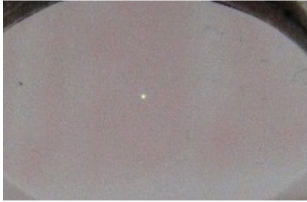
Figure 17: Sensor spot visible on the mirror.
