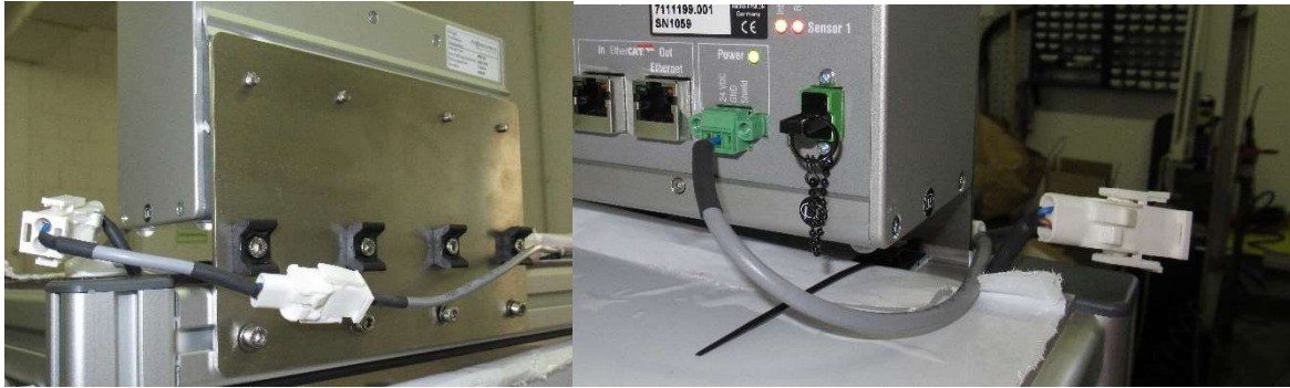
Figure 5: Left: Y-cable connected to 24 supply and to the fan, right: Connection to controller
