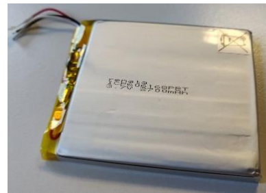
Figure 1. Lithium ion battery pouch cell tested herein.
